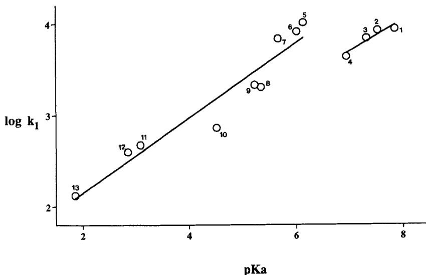
FIGURE 2 Brønsted plot of  $\log k_1$  vs  $\text{pK}_a$  ( $\text{H}_2\text{O}$ ) for the addition of substituted pyridines and imidazoles to  $[\text{Fe}(\text{CO}_3)(1\text{-}5\text{-}\eta\text{-C}_6\text{H}_7)]^+$  in  $\text{CH}_3\text{CN}$  at  $0^\circ\text{C}$ : 1, 2-MeIm; 2, 4-MeIm; 3, *N*-MeIm; 4, Im; 5, 3,5-Me<sub>2</sub>py; 6, 4-Mepy; 7, 3-Mepy; 8, 4-Phpy; 9, py; 10, 4-CHOpy; 11, 3-Brpy; 12, 3-CO<sub>2</sub>Mepy; 13, 4-CNpy.
